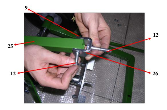
Secure the agitator to the reduction gear using screw (12) and nut (9).
