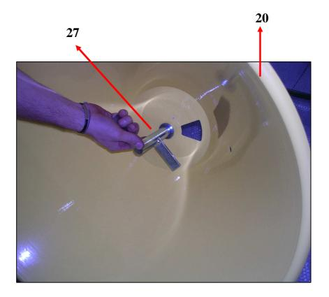
Then set the agitator (27) in the spreader disk as shown in the figure.
