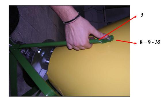
At this point, take the lever (32) and install the knob (33) and washer (34). Then secure the lever to the gate using screw (8) and nut (9).
