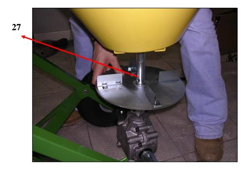
At this point, with the hopper set on the disk, install screw (12) which was previously set with hook (26) and nut (9).
