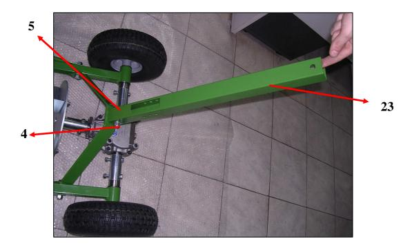
Secure the tow hook (24) on the draw bar (23) using the same screw (4) and nut (5).
