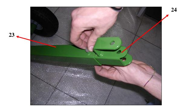
Take the strut (25) and install on the draw bar (23) using screw (12) and nut (9). Make certain that the furthest holes are closer to the draw bar (23).
