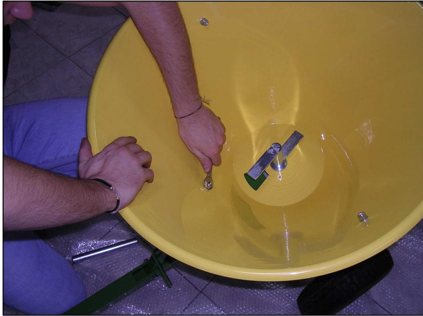
then the side screws (8) and the hopper shaft support screws (4).
