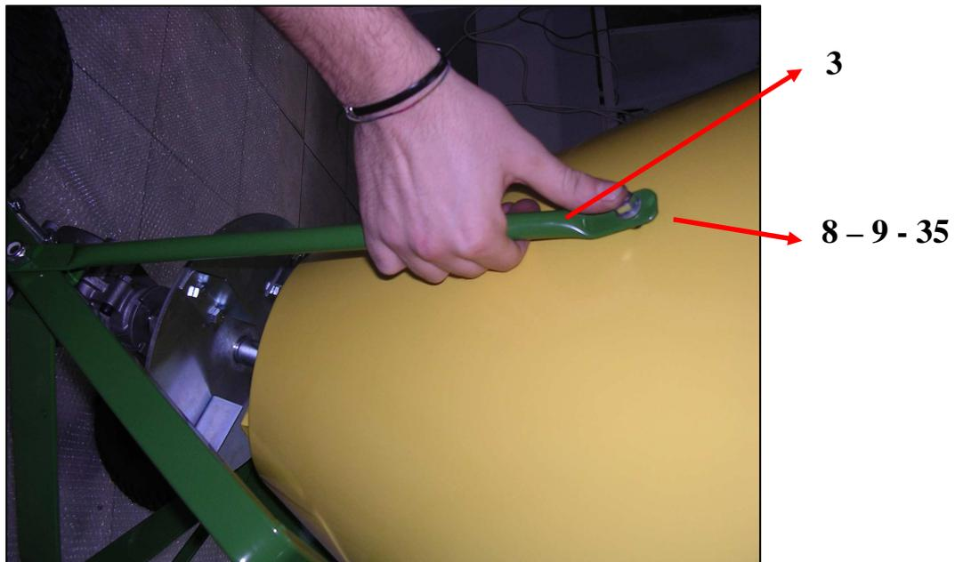
Secure the agitator to the reduction gear using screw (12) and nut (9).
