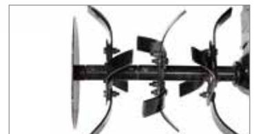
85 cm rotor with lateral protection discs.
